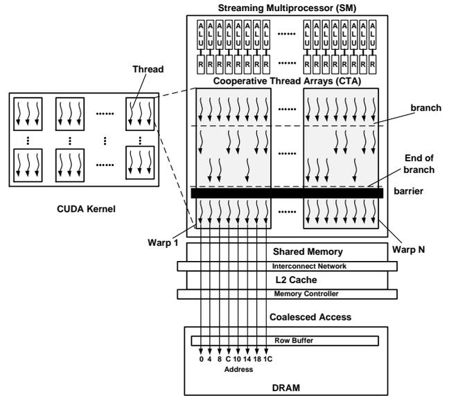
Figure 1: NVIDIA GPU Architecture and Execution Model.
